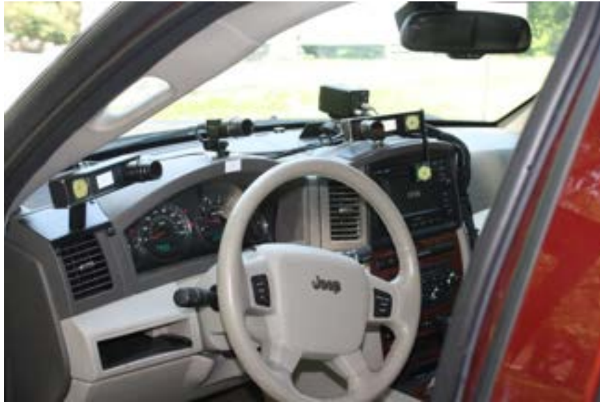
Figure 1. Eye tracking system camera placement.
