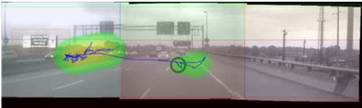
Figure 37. Heat map at end of fixations to CEVMS with long dwell time.
